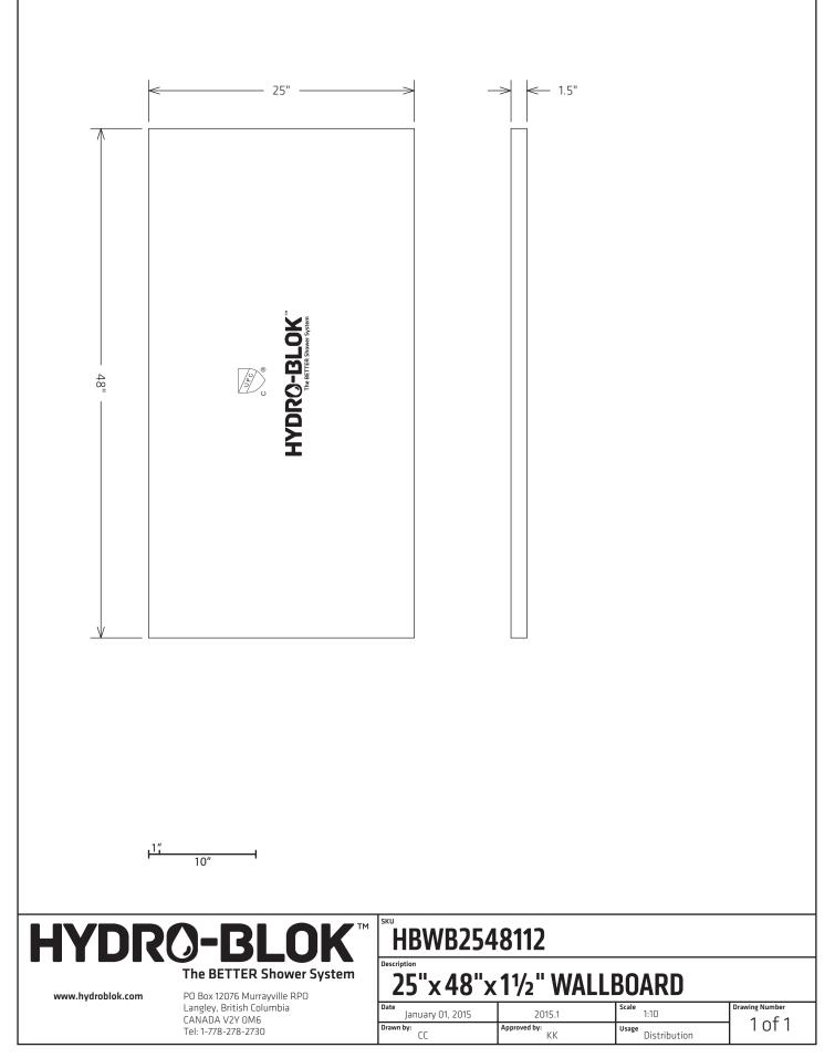
Disclaimer: Dimensional drawings are provided on an "AS IS" basis for planning and estimation only and are subject to change without notice. While reasonable efforts have been taken to ensure the accuracy of all dimensions, HYDROBLOK International Ltd. makes no warranties as to the completeness or accuracy of this document.
